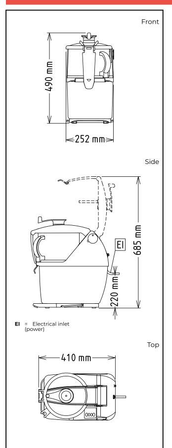
Electric Supply voltage: 200-240 V/1N ph/50/60 Hz Electrical power, max: 1 kW **Total Watts:** 1 kW Capacity: Performance (up to): 550 kg/Cycle **Capacity:** 4.5 litres Key Information: External dimensions, Width: 252 mm External dimensions, 485 mm Depth: External dimensions, Height: 505 mm **Shipping weight:** 30 kg
